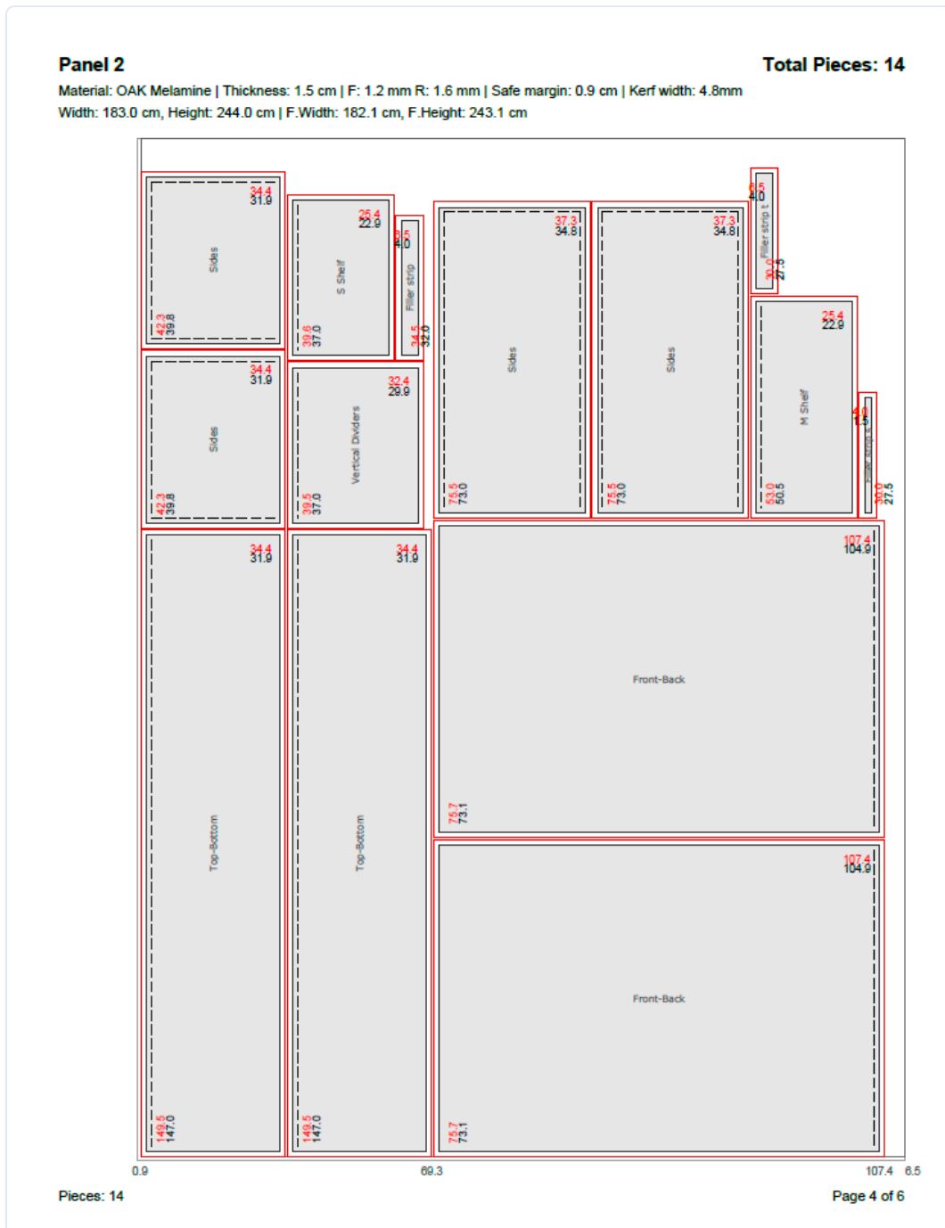
PDF nesting layout showing Panel 2 with part outlines, edgeband marks (red = rigid), dimensions, and part names.
